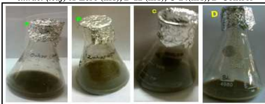
Figure No.4: Synthesis of silver nanoparticles from Anisomeles malabarica crude extract (boiled leaf) A-Zero (hrs), B-12 (hrs), C-24(hrs), D-Control
