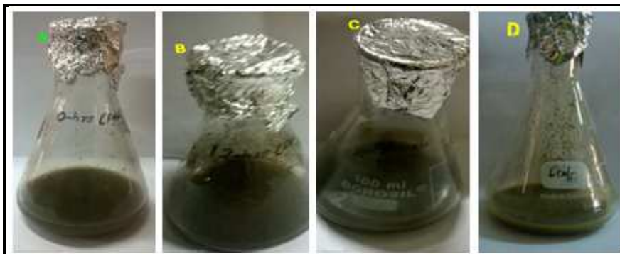
Figure No.3: Synthesis of silver nanoparticles from Anisomeles malabarica crude extract (leaf) A-Zero (hrs), B-12 (hrs), C-24(hrs), D-Control
