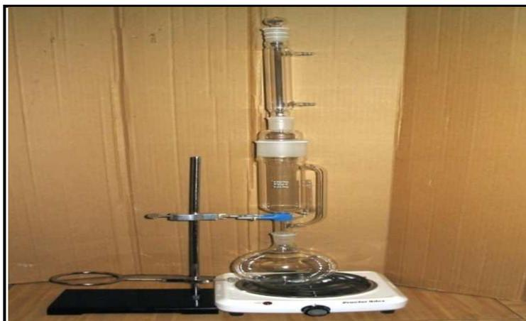
Figure No.5: Soxhlet Apparatus
